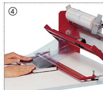
Slightly tighten the film and cut it off with the built-in knife.
